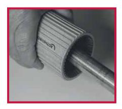
2. Debut tube both internally and externally to prevent damage to the fitting seal on assembly.
