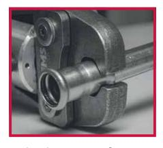
5. Place the correct press fitting jaw into the machine and insert the fastening bolt. Open the jaw at right angles to the fitting and activate the machine to pressfit.
