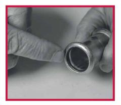
3. Ensure that the fitting O-ring is seated correctly. Add a small amount of appropriate lubricant to the O-ring if required.
