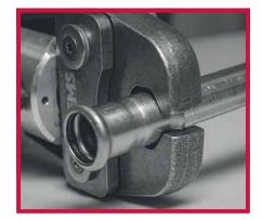
5. Place the correct press fitting jaw into the machine and insert the fastening bolt. Open the jaw at right angles to the fitting and activate the machine to pressfit.
