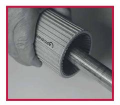
2. Debur tube both internally and externally to prevent damage to the fitting seal on assembly.
