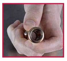
3. Ensure that the fitting O-ring is seated correctly. Add a small amount of appropriate lubricant to the O-ring if required.
