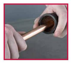
2. Deburr tube both internally and externally to prevent damage to the fitting seal on assembly.
